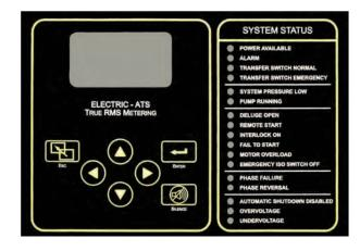
Description-Firetrol® FTA1350 Wye-Delta, Closed Transition Starting Fire Pump Controllers are used with delta-wound squirrel cage motors. FTA1350 controllers are of the closed circuit transition type in which the motor circuit remains closed during the transition from start to run. The controller monitors, displays and records fire pump system information.
